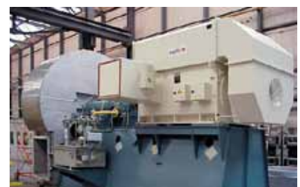
2600 kW vapour compressor for the sugar industry
